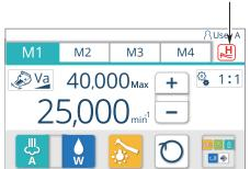
If the product is used for a long time at a high load, the overheating prevention function is activated and the torque is automatically decreased, in order to prevent the micromotor unit overheating. If this occurs, a buzzer sound is heard, and  $extrm{H}$  is displayed. While this indication is displayed, the overheating prevention function is activated.
