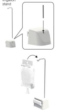
2. Insert the irrigation stand into the hole on the back of the pump cover.
