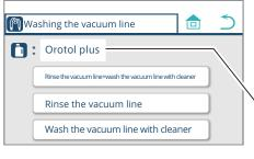
\* If you select 'Washing the vacuum line', the amount of remaining cleaner will be checked. If the amount of cleaner is sufficient, the screen shown in the left figure appears.
