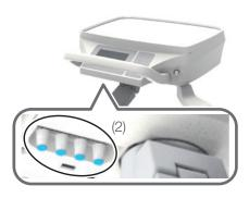
Adjusting the quantity of water supplied to the handpiece spray
