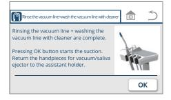
3. When you have finished rinsing the vacuum line+washing the vacuum line with cleaner, press the ok switch.
