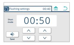
6. Press Store Switch to save the setting The flushing screen in 3. appears.
