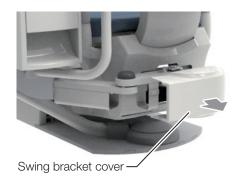
7. Remove the swing bracket cover by pulling in the direction of the arrow. Pull up the lock lever A and turn it until the lever is locked in place.
