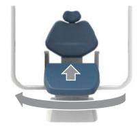
3. After moving the light pole, adjust the position of the balance arm to position as shown on the left figure.
