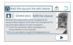
\* If the amount of cleaner is insufficient, the screen shown in the left figure appears. Refill the cleaner.
