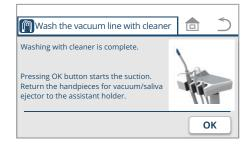
3. When you have finished washing the vacuum line with cleaner, press the  $o\kappa$  switch.
