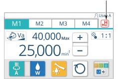
If the product is used for a long time at a high load, the overheating prevention function is activated and the torque is automatically decreased, in order to prevent the micromotor unit overheating. If this occurs, a buzzer sound is heard, and  $\checkmark$  is displayed. While this indication is displayed, the overheating prevention function is activated.
