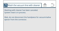
\* If the x switch is pressed during washing, the screen shown in the left figure appears.
