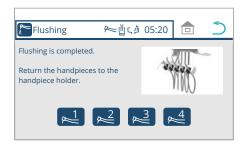
7. Once flushing is completed, return the handpiece to the instrument holder. When the handpiece is returned, the home screen appears.
