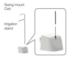
2. Insert the irrigation stand into the hole on the back of the pump cover.
