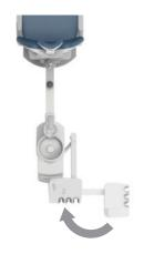
9. Switch the position of the assistant holder to the other side. At that time, the vacuum hose and saliva ejector hose will twist. Pick them up from the assistant holder to remove the twist.
