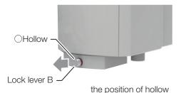
11. Turn the lock lever B so the hollow comes to the downside position. The lock lever B may not return to lock position. In that case, adjust the position of the cuspidor body until the lock lever B is back in lock position.
