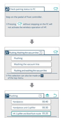
Hold down the pedal of the wireless foot controller until the flushing screen appears.
