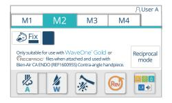
In reciprocal mode, the micromotor oscillates at preset angle, acceleration speed, and torque value.
