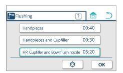
4. Check "HP, Cupfiller and Bowl flush nozzle 05:20" is selected and press ok switch.
