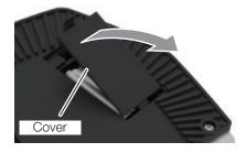
3. Insert two new/charged AA batteries into each box. Use alkali dry batteries or NiMH batteries.
