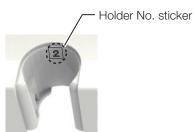
Each holder sleeve has its No. on the bottom, and a sticker showing the same No. is attached to the assistant holder.
