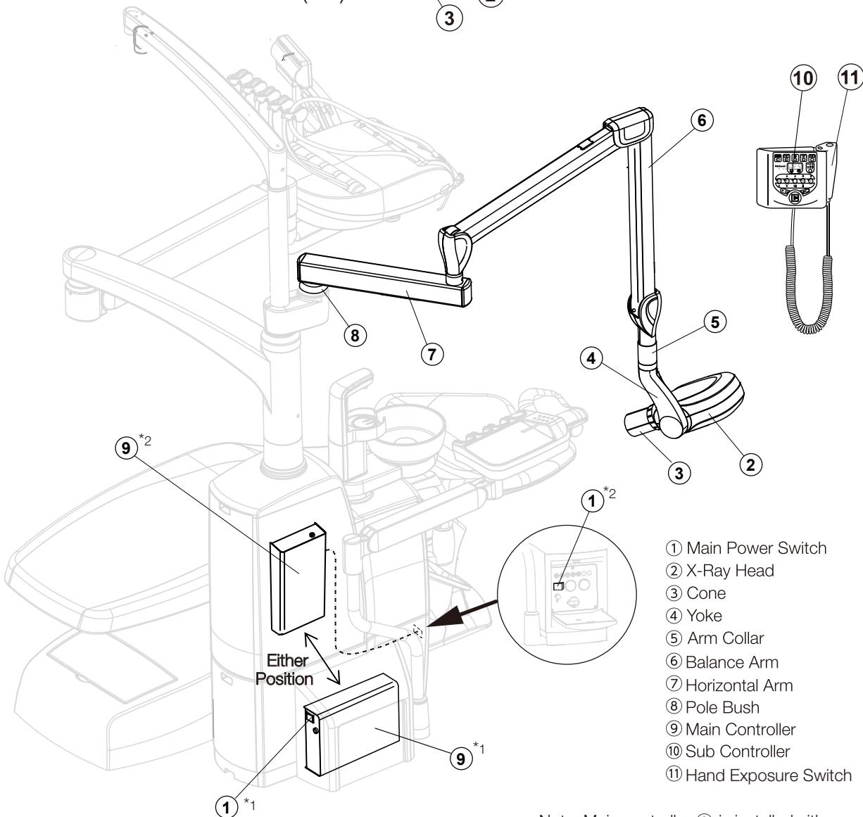
Note: Main controller ⑨ is installed either outside (\*1) or inside (\*2) of the dental unit.
