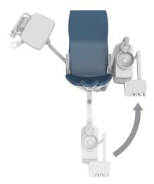
10. Swing the cuspidor unit and the assistant holder as shown on the left figure. When the cuspidor unit reaches the correct position as shown on the left figure, the lock lever A on the swing bracket will lock automatically.
