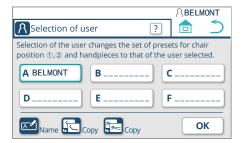
In this example, the name "BELMONT" has been entered. The registered name is indicated for the User memory A box and displayed at the top right.
