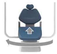
3. Lift the toe board of the seat cushion and swing the light pole to the other side as shown on the left figure.
