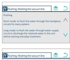
Explanation of flushing and washing the vacuum line
