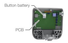
2. Detach the button battery (CR1632) on the PCB.
