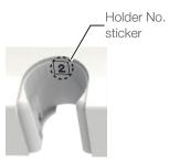
Each holder sleeve has its No. on the bottom, and a sticker showing the same No. is attached to the assistant holder.
