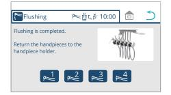
7. After rinsing of the vacuum line is completed, return the handpieces for doctor unit to the instrument holder.
