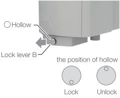
12. Turn the lock lever B so the hollow comes to the downside position.
