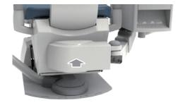
12. Attach the swing bracket cover to the swing bracket.
