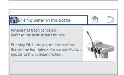
9. In the event of an error state, take appropriate measures. In the event of an error state before/upon/during washing with cleaner/rinsing, the system will be reset and the error screen will appear.
