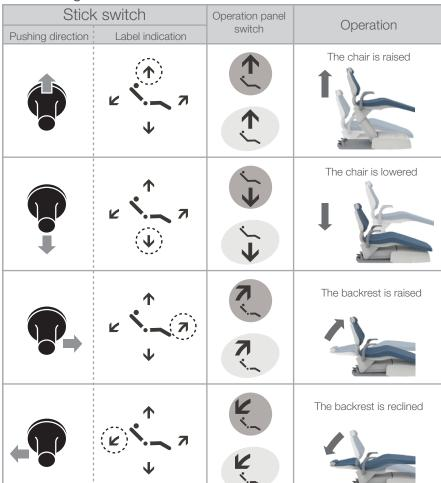
\*The chair is operated while the stick switch is pushed down or the switch is pressed.
