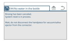
4. In the event of an error state, take appropriate measures. In the event of an error state before/upon/during washing with cleaner/rinsing, the system will be reset and the error screen will appear.
