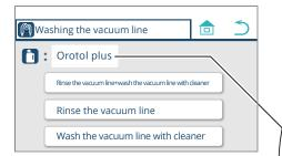
\* If you select 'Washing the vacuum line', the amount of remaining cleaner will be checked. If the amount of cleaner is sufficient, the screen shown in the left figure appears.
