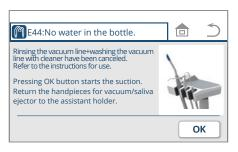
4. In the event of an error state, take appropriate measures. In the event of an error state before/upon/during washing with cleaner/rinsing, the system will be reset and the error screen will appear.
