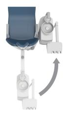
11. Swing the cuspidor unit and the assistant holder as shown on the left figure. When the cuspidor unit reaches the correct position as shown on the left figure, the lock lever A on the swing bracket will lock automatically.
