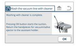
3. When you have finished washing the vacuum line with cleaner, press the ok switch.
