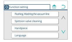
2. Press the 'Flushing, Washing the vacuum line' switch.
