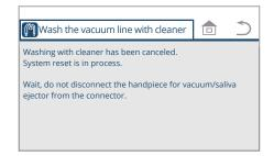
\* If the \_\_\_\_\_ switch is pressed during washing, the screen shown in the left figure appears.
