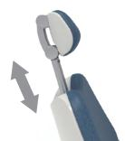
Do not apply excessive load or impact to the headrest while it is extended. Do not hit the headrest from above. Otherwise, failure may result.
