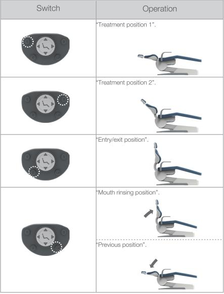
Do not press the stick switch for automatic operation for five seconds or longer. If pressed for five seconds or more, a buzzer sound is heard, and the chair position at that point is memorized as a preset position.
